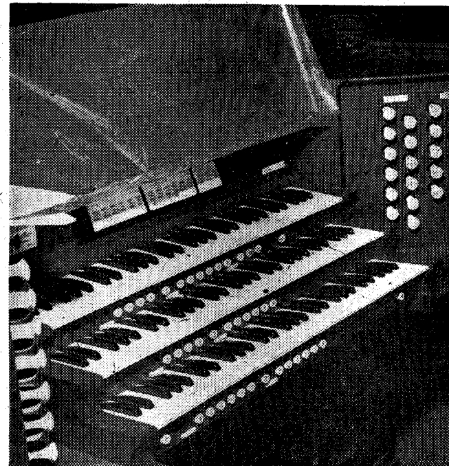
THREE MANUAL console of drawknob type is favored in all large installations. Many buttons below the manuals activate a remote control mechanism which changes combinations of stops.
