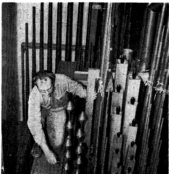
INSIDE ORGAN, an organ tuner checks an English Horn as the tonal designer works at the console. One of the reed stops, the English horns require the most delicate adjustment.
