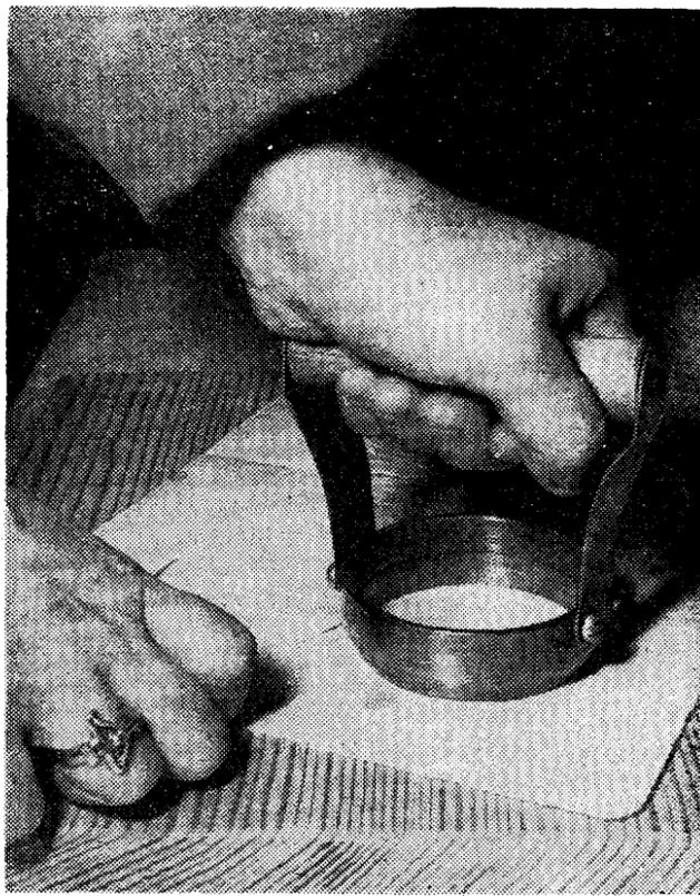
**Hand Press Is Used To Cut Out Large Hosts**
